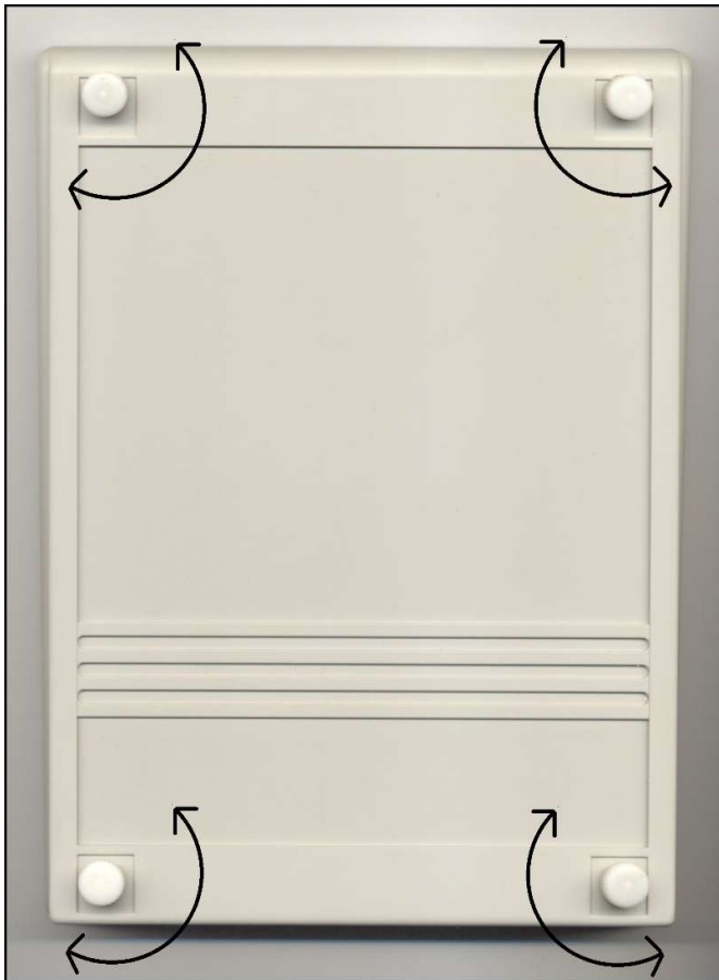
Figure: Opening the Emulator Box
