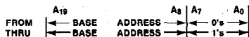
MEMORY DATA NEED NOT BE ALIGNED TO EVEN ADDRESS BOUNDARIES I/O TRANSFERS MUST BE WORD TRANSFERS TO EVEN ADDRESS BOUNDARIES
