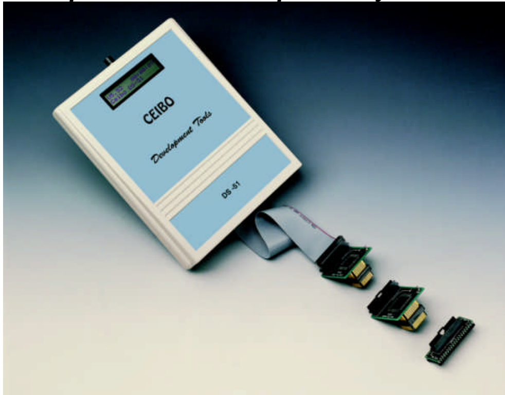
In-Circuit Emulator for 8051 Family of Microcontrollers
