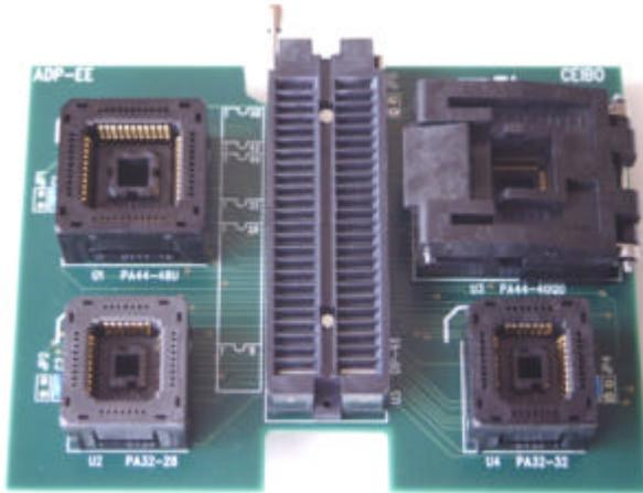
Universal programmer adapter. It connects 48 Dip to different sockets. The list of sockets on the adapter is:
